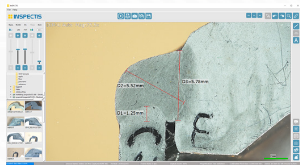
Weld bead inspection and measurements with INSPECTIS®
