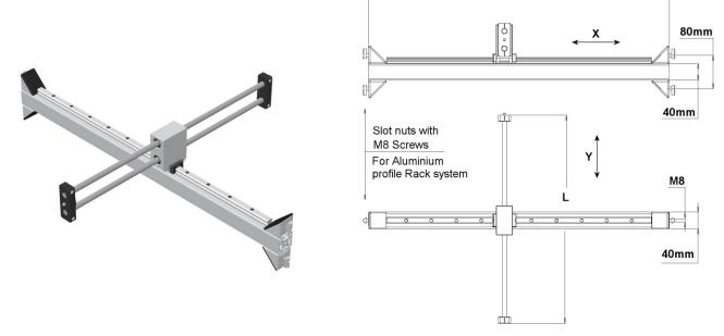
Custom cut linear guiding system mounted on high density aluminum profile for X-travel and a rigid custom sized double-arm boom creates requested Y-travel range of the Digital Microscope. The X profile is fitted with mounting brackets to allow the correct setting of working distance during installation in the user's rack system.
