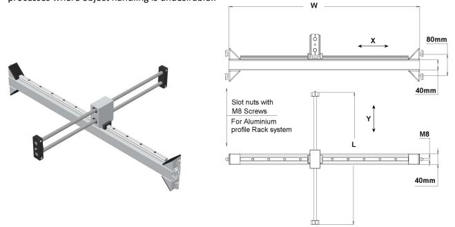
Custom cut linear guiding system mounted on high density aluminum profile for X-travel and a rigid custom sized double-arm boom creates requested Y-travel range of the Digital Microscope. The X profile is fitted with mounting brackets to allow the correct setting of working distance during installation in the user's rack system.
