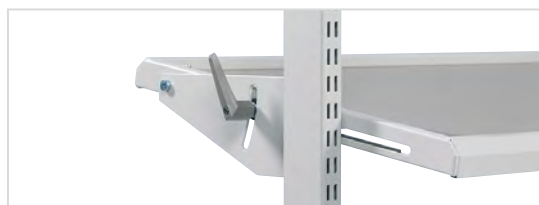
Steplessly adjustable shelf, tilting 0-25°
